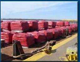
SlingBag® pallets are shipped with a weather resistant pallet cover and can be double stacked on off-shore vessel.
